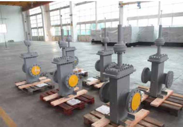
HG-1, 8" 400, soft seated, CS+ENP, impact test at -55°, onshore, Russia
