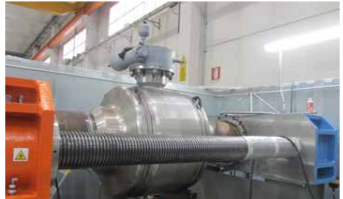
HB-3, 20" 1500, soft seated, CS/DSS, 100 cycles test, subsea, India.
