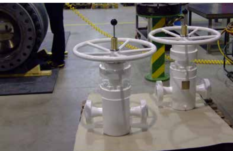
HG-1, 1" 13/16 API 10000, metal seated, CS/SS+TCC API 17D subsea, Gulf of Mexico
