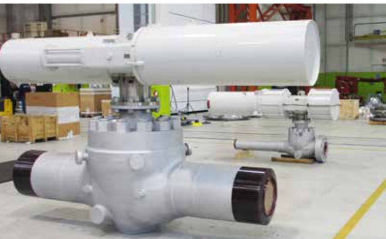
HB-2, 18"x14" 2500, metal seated, CS/DSS/SDSS c/w pup pieces 650 mm, DIB-1 tested offshore, Norway
