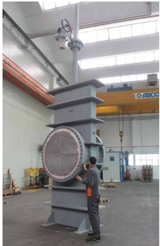
HG-3, 48" 600, metal seated, CS+ENP above-ground installation, Europe
