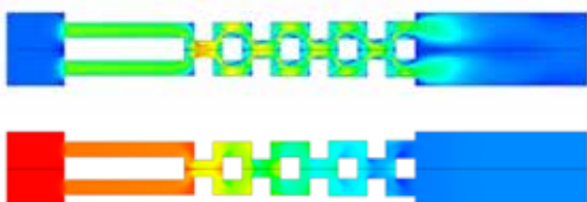
VELOCITY AND PRESSURE PROFILE ACROSS A TRIM LABYRINTH
